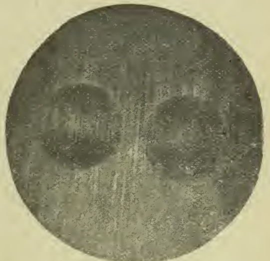
Fig. 6.—Brinell impression \times 20 .
